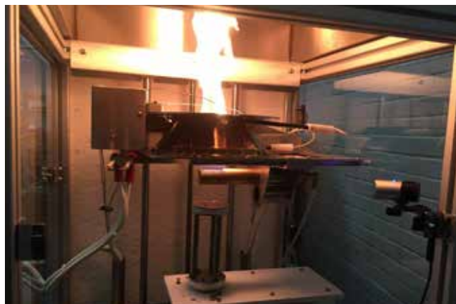
Test by cone calorimeter as refer to ASTM E1354:2017
